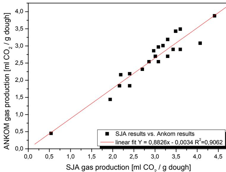
Fig. 7: Overall correlation for all doughs measured with both systems.
