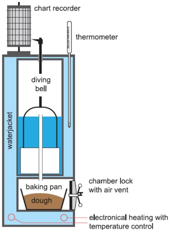
**Fig. 1:** SJA Fermentograph in principle
