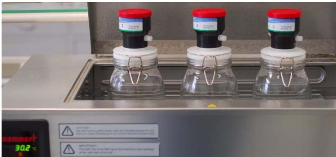
**Fig. 2:** Experimental set up for dough testing at the VH Berlin using ANKOM pressure measurement modules with prototype adapters connected to 1.85 L glass jars.
