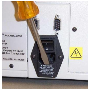
Pry the fuse holder out of the On/Off switch
