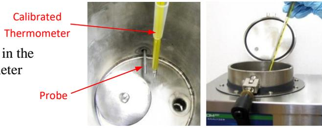
8. Record the readings on the thermometer and on Display 1. Repeat two additional times during the heat-up.
